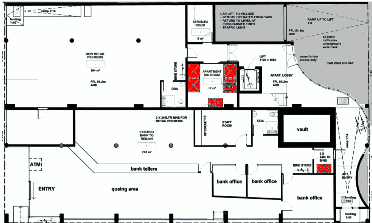
GND Retail space (164 sq m), bank (280 sq m), BINS, car lift to level 1 a car stackers
